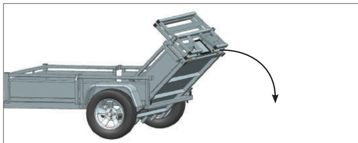
Figure 18: Trailer unfolded with hitch pins in position
